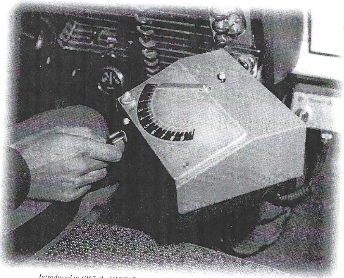
Introduced in 1967, the VASCAR speed-measurement device allowed troopers to clock vehicles moving in either direction in all kinds of weather. (Courtesy MSP Photo Lab)
